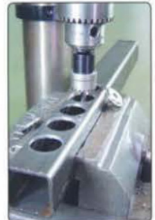
Square pipe boring
