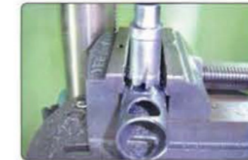
Stainless steel pipe boring
