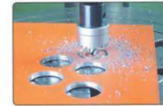
Steel plate boring
