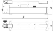
P-series hydraulic hand pumps are designed for Cylinder and hydraulic bolt tensioner. Its pressure anew to two types(70Mpa & 160Mpa), and customers can order every size of oil tank for different equipment. KANAZAWA serves a wide range accessory for this series. These products which are designed for serving true resolutions, entitled with TUV seal result of an effort with appropriate directives.
