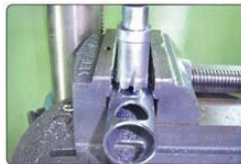
Stainless steel pipe boring
