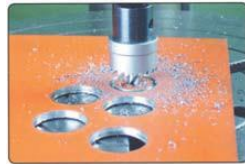
Steel plate boring
